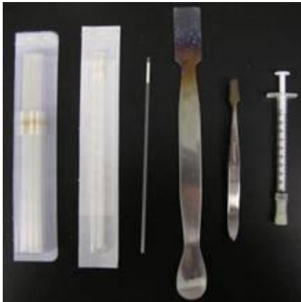
0.25 ml Straw 133 mm * 1.6 mm (ID) Ionomer resin (cryo bio system)
